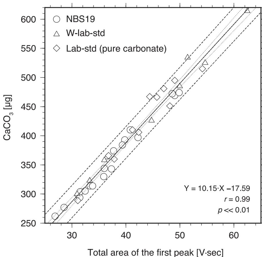
Figure 8: Scatter diagram showing CaCO<sub>3</sub> [µg] reacted with phosphoric acid and total area [V·sec] of the first sample aliquot peak (sum of areas of mass 44, 45, and 46) (cf. Figure 2). Solid, dotted, and dashed lines show the least-squares regression, 95 % confidential interval, and 95 % prediction interval for the regression, respectively.
