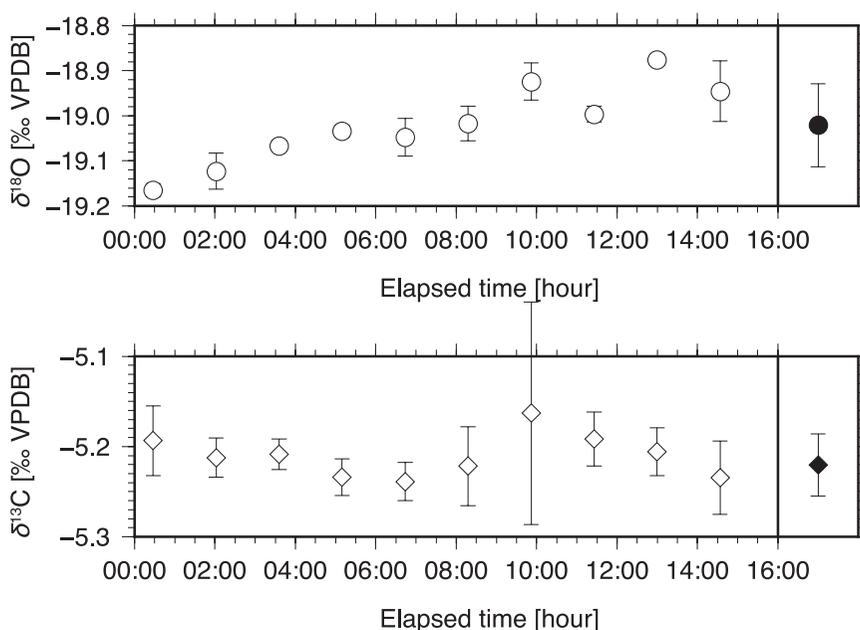
Figure 7: Time series analyses of the Lab-std (pure carbonate) over 16 consecutive hours. Open symbols and whiskers show average and standard deviation ( $1\sigma$ ) of quadruplicate aliquots analyses of each sample (cf. Figure 2). Filled symbols and whiskers show average and standard deviation ( $1\sigma$ ) of all analyses. Note that y-axis scale is different from the other figures.
