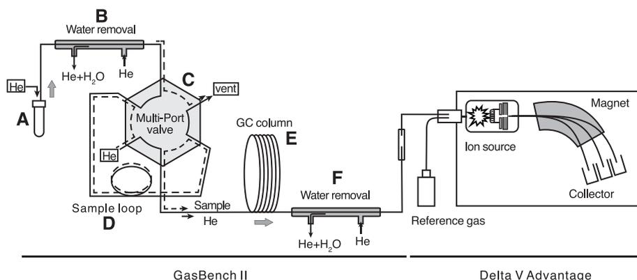
Figure 1: Schematic diagram showing GasBench II inlet system and Delta V Advantage mass spectrometer. A. Autosampler (96 vials); B. Water removal system 1; C. Loop injection system; D. 100  $\mu\text{l}$  sample loop; E. Isothermal gas chromatograph; F. Water removal system 2.
