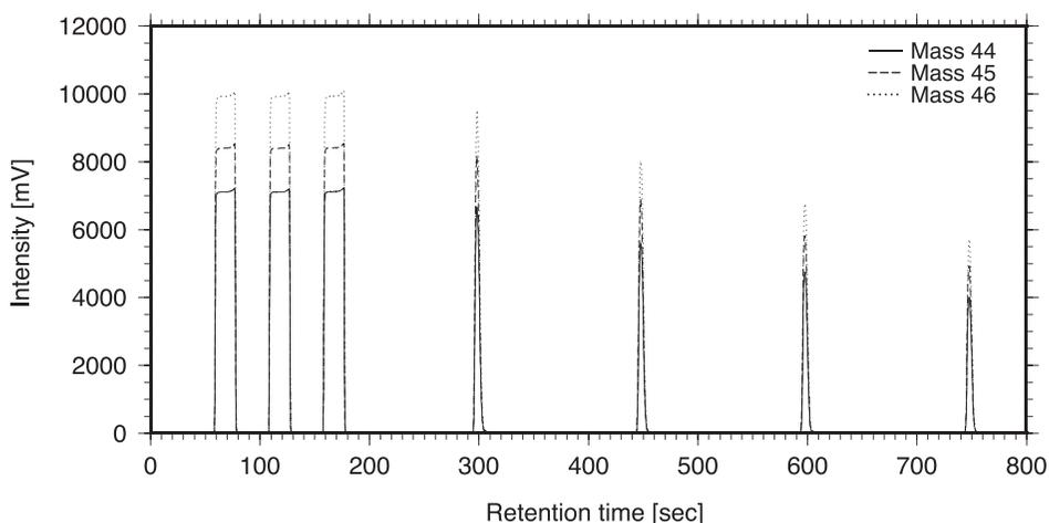
Figure 2: Typical chromatogram of  $\text{CO}_2$  isotope ratio analysis. Three reference gas injection pulses at 70, 120, and 170 sec are followed by a set of four sample gas aliquots pulses at 300, 450, 600, and 750 sec for each sample.
