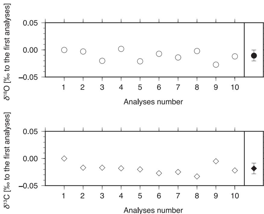
Figure 3: Carbon and oxygen isotope ratios of multiple analyses of online reference  $\text{CO}_2$  gas showing the internal precision of Delta V Advantage in our laboratory. Open symbols show each reference gas analysis. Filled symbols and whiskers show average and standard deviation ( $1\sigma$ ) of 10 consecutive analyses, respectively.
