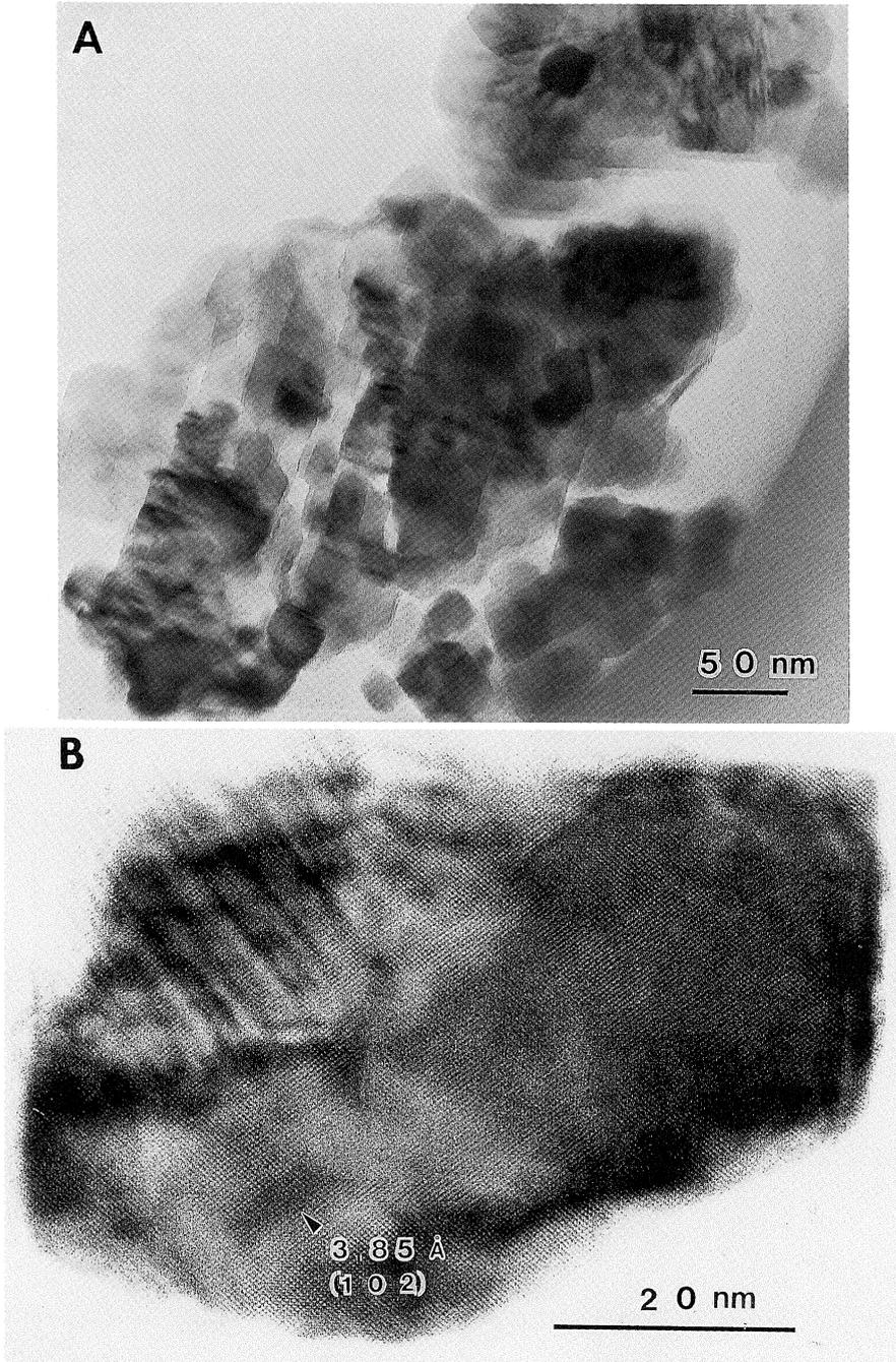
Fig. 13. Transmission electron micrographs of the dinosaur eggshell sample 2; RTMP 87. 79.85. A; mosaic structure of calcite, B; higher magnification of A showing lattice images of calcite  $3.85 \text{ \AA}$  (1 0 2) d-spacing with lamellar deformation features.
