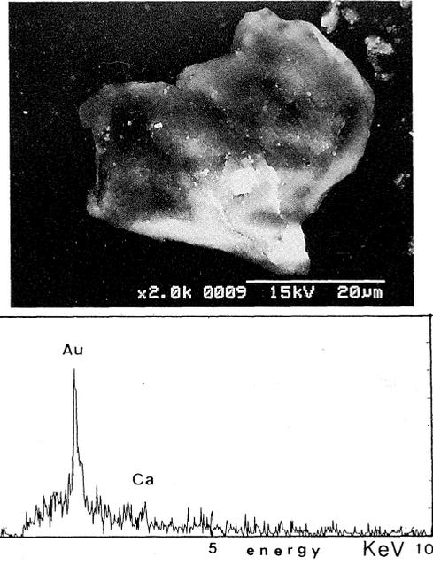
Fig. 11. Scanning electron micrograph of organic materials of membrane and its EDX from the powdered sample 2; RTMP 87.79.85. Strong peak of Au is due to ion-spattered coating material whereas small Ca peak is due to calcite grain on the surface.
