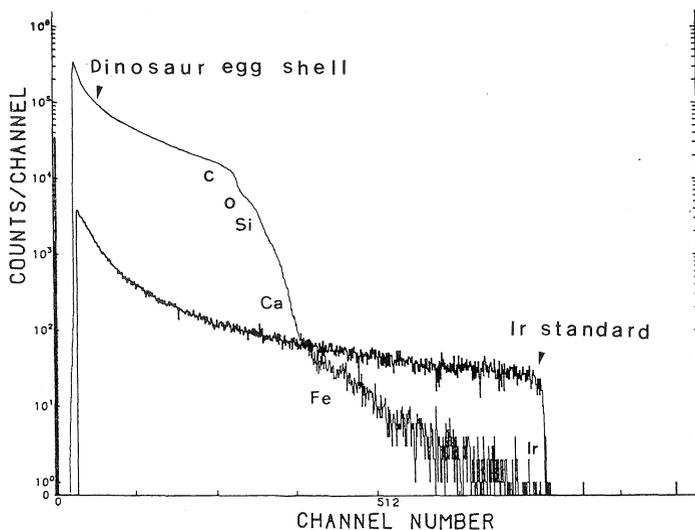
Fig. 14. Energy spectra by heavy ion probe Rutherford scattering for the dinosaur eggshell sample 1; RTMP 86.49.15 in comparison with iridium standard sample. The eggshell mainly composed of C, O, Si, Ca, Fe and a trace of Ir.
