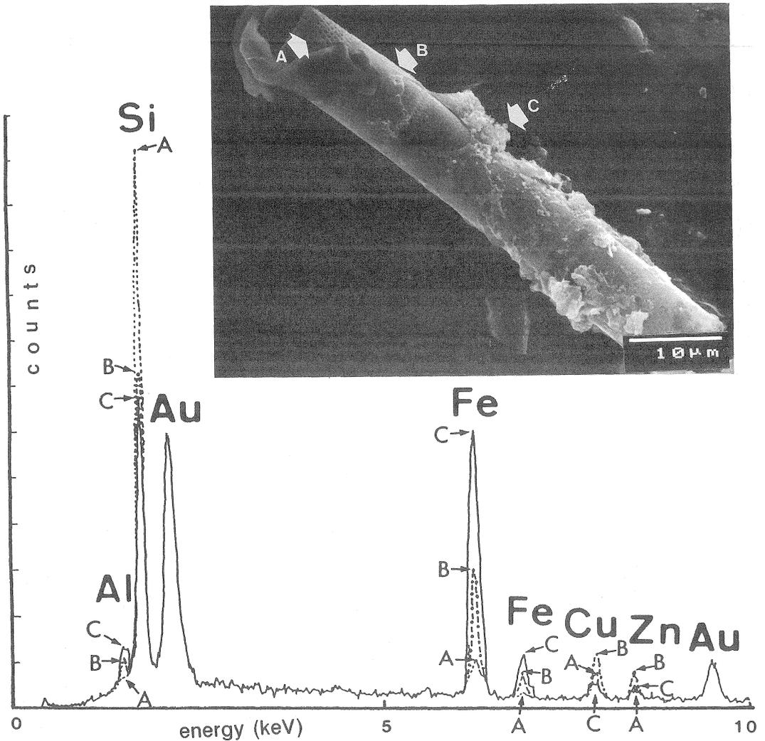
Fig. 7 SEM-EDX of *Aulacoseira sp.* showing three different compositional steps. The EDX data indicate Si, Fe and Al deposition of the diatoms' valve (A), a thin film which covers the valve (B) and the minerals' aggregates (C).
