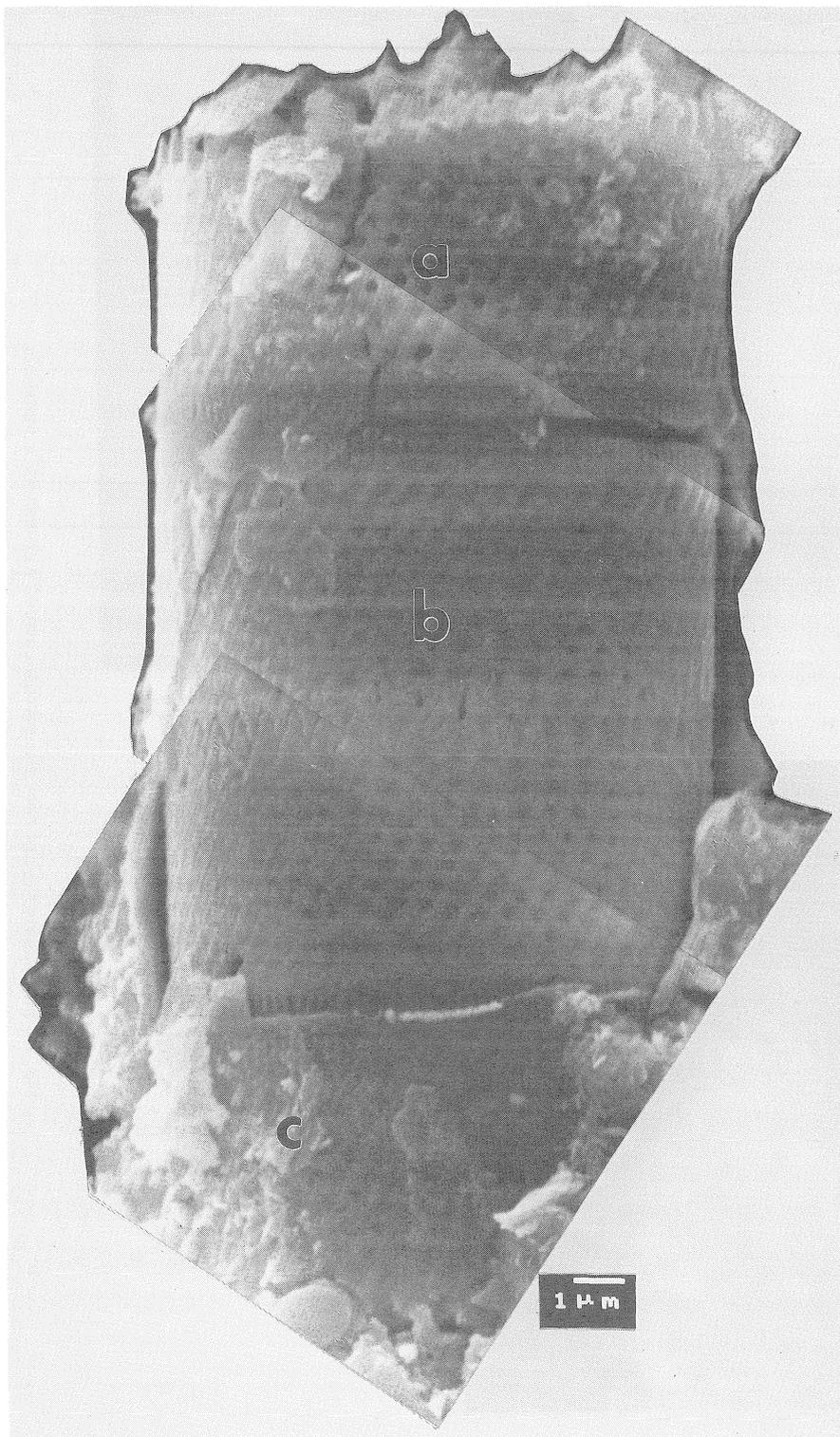
Fig. 5 SEM micrograph of *Aulacoseira* sp. covered with mineralic films. (a) the own diatom valve, (b) the smooth film and (c) the aggregate film.
