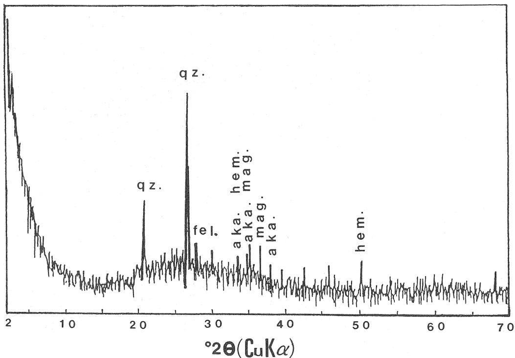
Fig. 2 The XRD results from the sample where the diatoms were found. qz.; quartz, fel.; feldspar, hem.; hematite, aka.; akaganeite, mag.; magnetite.
