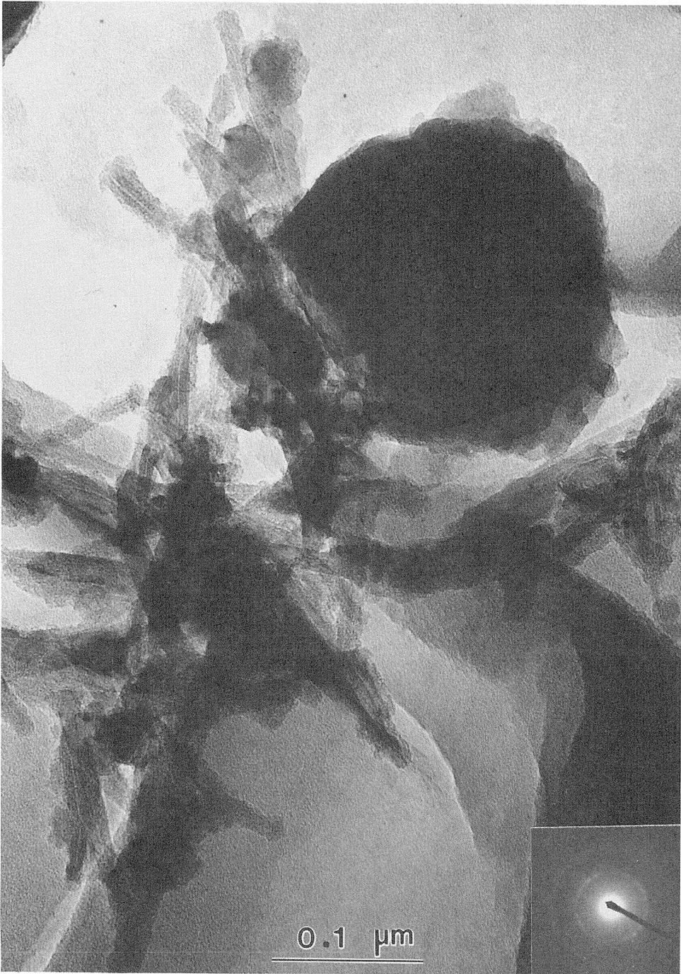
Fig. 7. Transmission electron micrograph of hematite blades associated with coccoid bacterial cell. The electron diffraction (inset) shows spots at 2.56, 2.47 and 1.70 Å.
